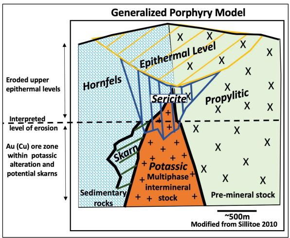
Figure 8-1: Generalized Porphyry Model Cerro de Oro
