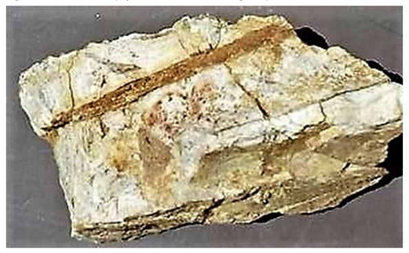
Figure 7-7: Altered Porphyritic Granodiorite with High Sulphide Content
