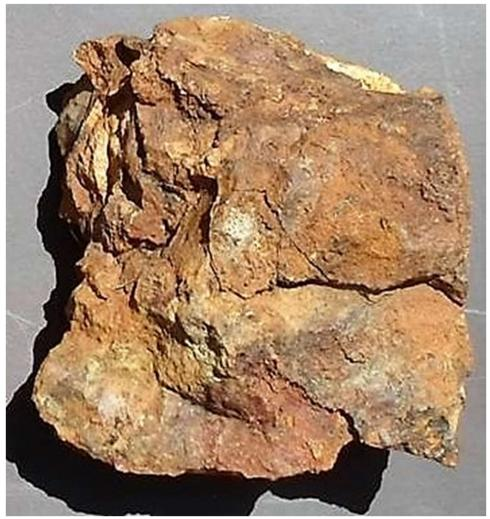
Figure 7-10: Sericitically Altered and Silicified Calcareous Siltstone of Caracol Formation
