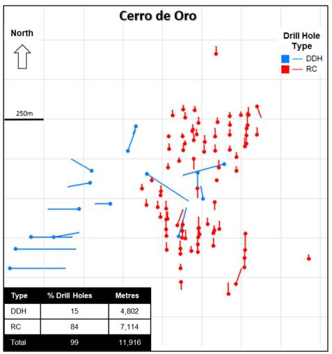
Figure 14-1: Drill Holes Used for 2020 Mineral Resource Estimation
