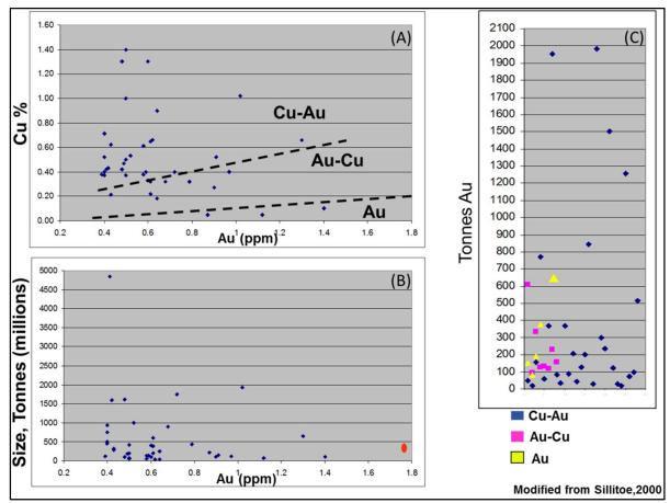
Figure 8-2: Classification of the Three Gold-Rich Porphyry Systems
