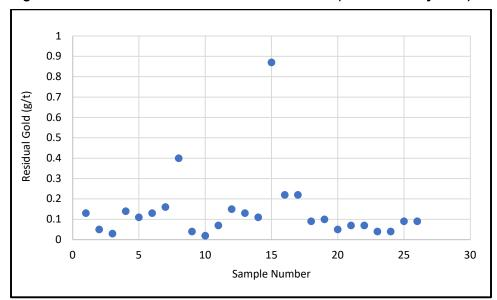
Figure 13-12: Gold Content in Leach Test Residues (SGS—January 2019)
