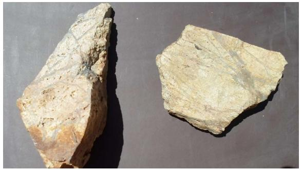
Figure 7-6: Examples of Stockwork Quartz Veining in the Porphyritic Granodiorite Intrusive
