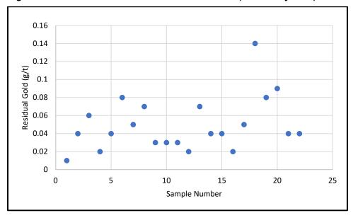
Figure 13-7: Gold Content in Leach Test Residues (SGS—July 2018)
