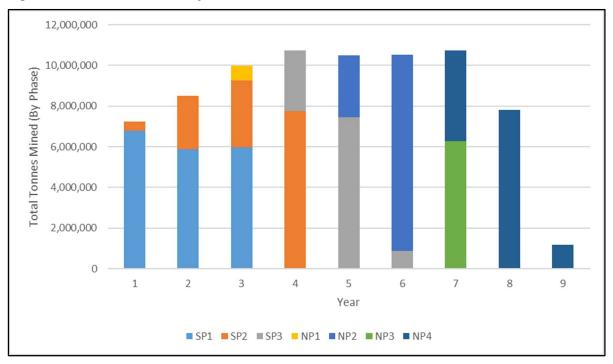
Figure 16-4: Material Mined by Phase
