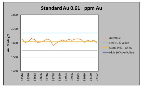
Figure 11-2: Standard Assay Results (0.61 g/t Au)
