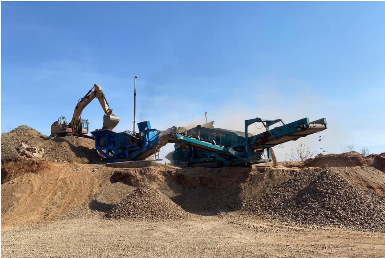
**Photo 2 – Portable crushing equipment in action opening up the Nicho Norte open pit.**
